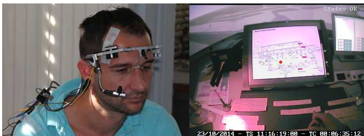
Figure 1: (left) Electrocardiogram (not pictured), electroencephalogram, and eyetracker installed on a participant. (right) View from eyetracker forward-facing camera.
