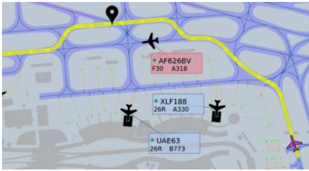
Figure 2: Standard route modification using waypoints.
